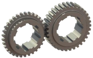
Test geometry pitting
