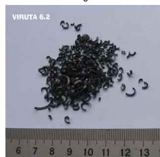
Chip morphology generated during external turning - 40CrMoB4
